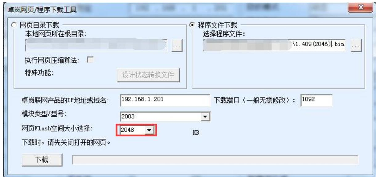
picture58 LAN2003Firmware upgrade method
